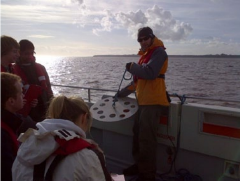
Figure 2: Students preparing to deploy an underwater sonar calibration plate
