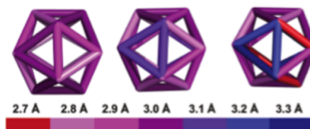
Figure 1. A 'heat map' showing evolution of bond lengths of the icosahedral core of \text{Au}_{25}(\text{SR})_{18} in three oxidation states, increasing from negative to positive from left to right.
