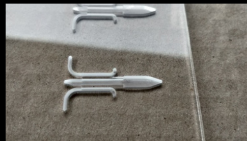
Prototype microfluidic chip generated using micro-milling techniques. Image: FPC@DCU
